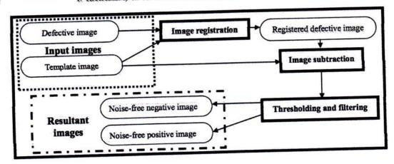
FIGURE 3. Flow process of the inspection algorithm
