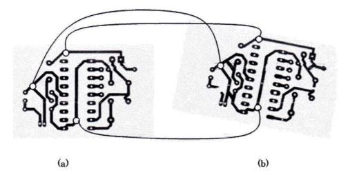
FIGURE 2. (a) Template image; (b) defective image (rotated by some degrees)
