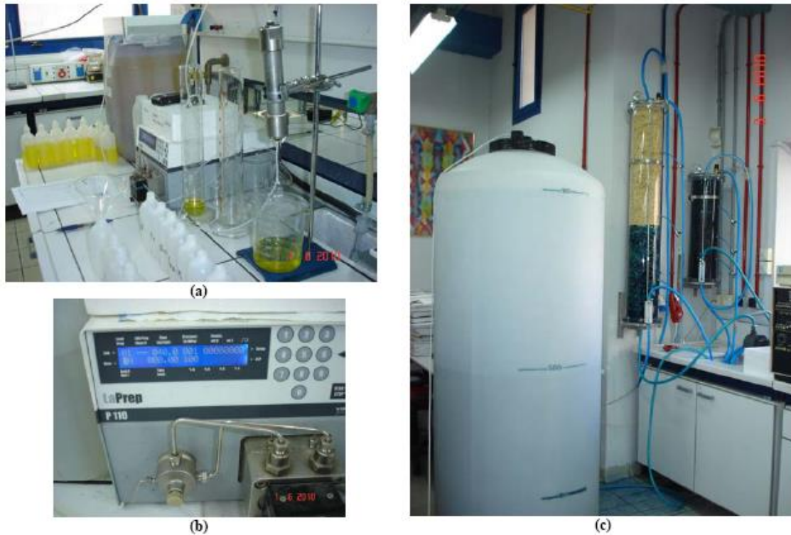
FIGURE 2. (a) Laboratory scale column of 15 cm height with 25 L tank, (b) laboratory scale pump, and (c) pilot scale column of 137 cm height with 1000 L tank.
