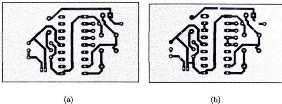
FIGURE 1. (a) A template bare PCB image; (b) a defective bare PCB image
